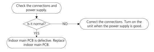
Note: E2 zero crossing detection error is only valid for the unit with AC fan motor, for other models, this error is invalid.
